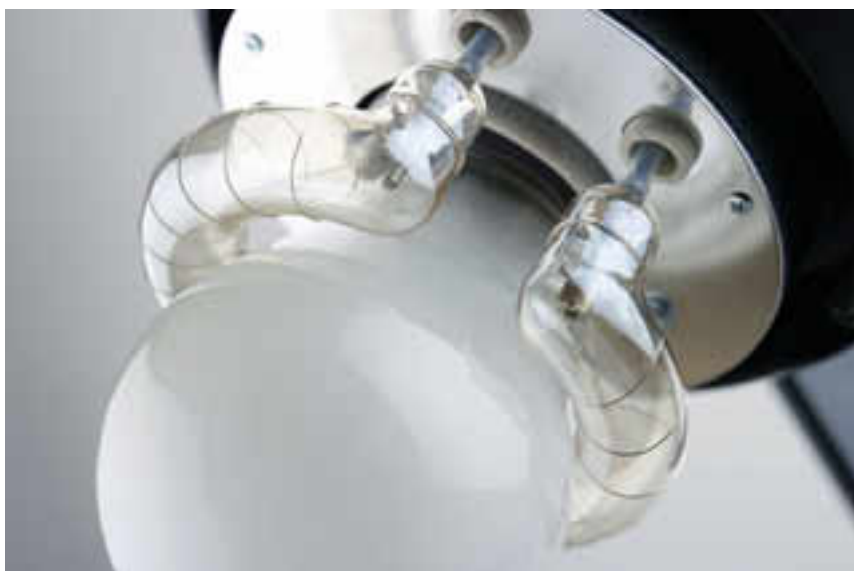
A typical bare flash tube without any accessories is largely a useless light source.
