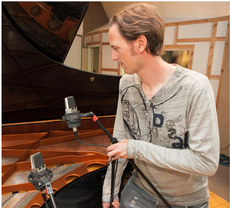
In order to give better audibility of the piano's higher register, the instrument's spot microphones were moved lower down, bringing them closer to the upper strings.
