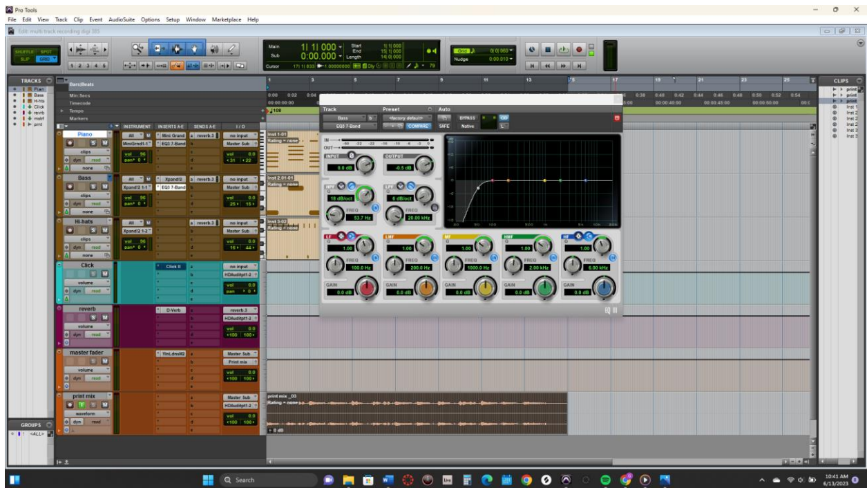
Bass and Hi-Hats EQ set up. I only used a HPF at 53.7 Hz
