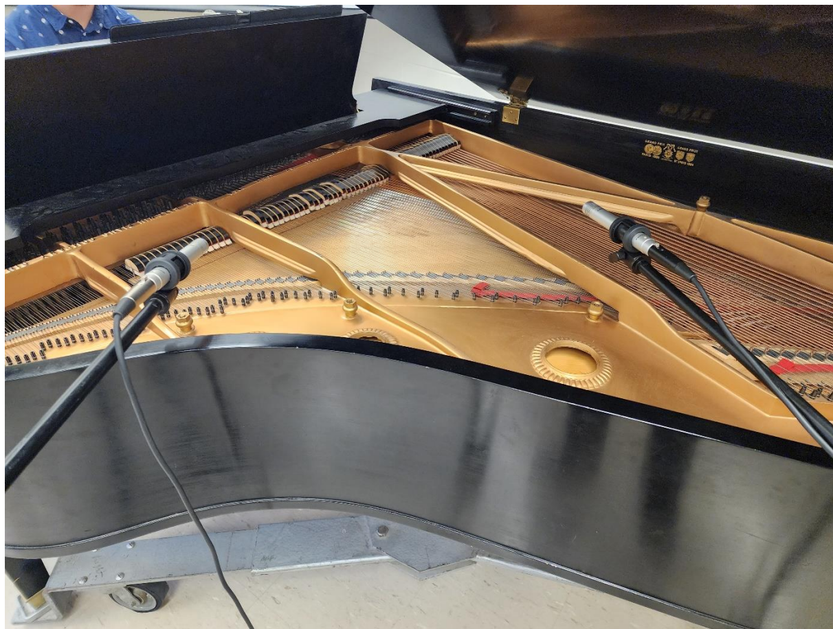
Picture 3: Spaced pair mic set up the right mic pointed towards the bass while the other is pointed towards the hi mids.
